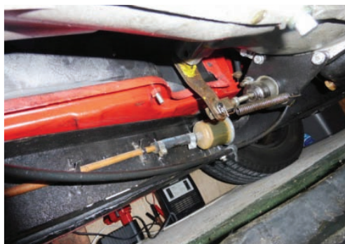
Mechanical fuel filter blanking plate studs are used to support fuel line.
